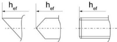
Alternative point geometry threaded rod RGM
